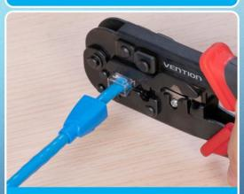
5. Buckle the RJ45 strain relief boots onto the RJ45 plug, put it into the crimping tool to press the interface, and push it into place for crimping
