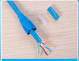
2. Subtract the cross frame and anti-drawing in the network cable (ignore if do not have one)
