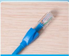
4. Insert the flattened cable into the front part of the RJ45 plug
