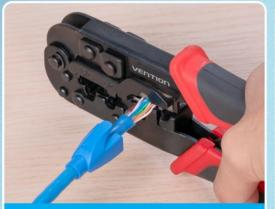
3. Arrange and cut the cables accordingly (in the sequence of 568A/B) (reserve about 1.5cm)
