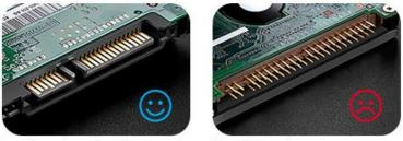
SATA (serial) interface Supported IDE (parallel port) interface Not supported
