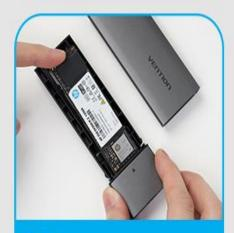
Fasten the black fastener to fix the SSD
